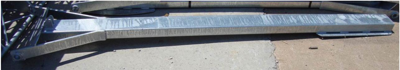
3. Tail Boom: 145 lbs, 13" x 114" x 24" (HxWxD)
